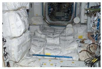
Figure2: ISS assets stowed in flight bags and secured to walls
