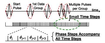
Figure 3: Global SAW Tag Data Encoding Example
