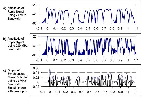
Figure 6: Pulse Response from 2.44 GHz Global SAW Tag with Pulses for Start, Stop, Synchronization, 64 Data Bits, and 16 Bit Error Detection. Uses Fundamental Mode Design on 128<sup>o</sup> LiNbO<sub>3</sub>
